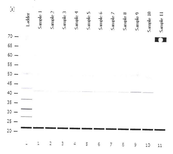
Samples 1-9 are the test swabs. Sample 10 is the negative control and sample 11 is the positive control.
